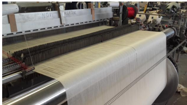
Image 4. Weaving on FIMTESSILE RP120
