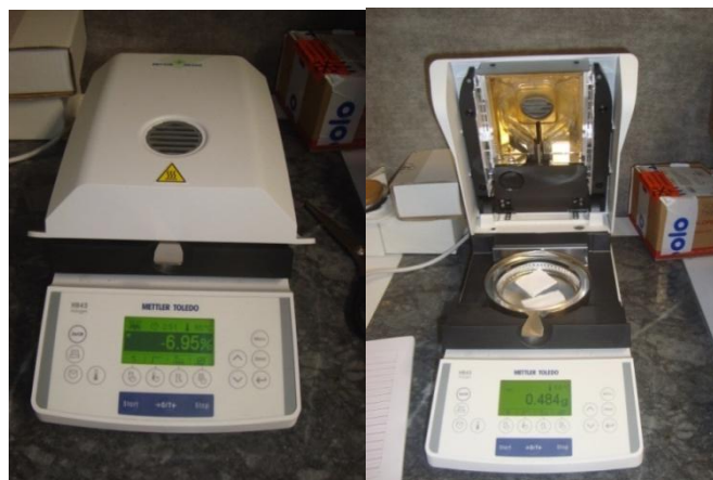
Figure 1. A device HB 43 (Mettler Toledo) for determination the moisture content of knitted fabrics
