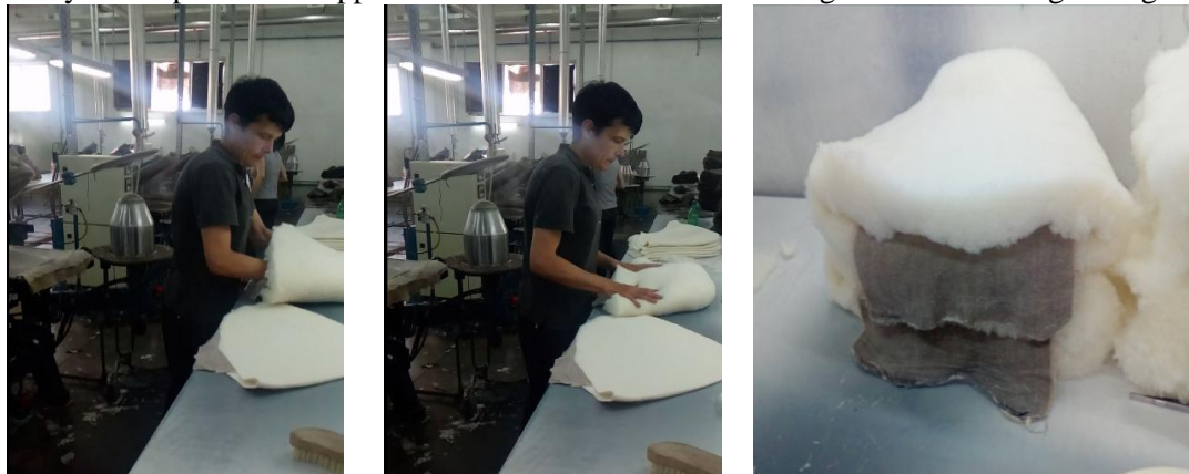
Pictures 18,19,20: Placing a patch inside the cone
