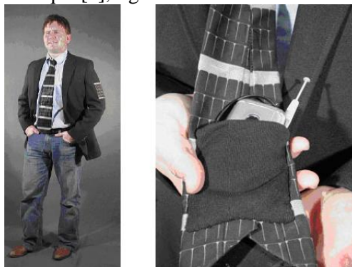
Figure 9. Photovoltaic tie made with satin fabric.
