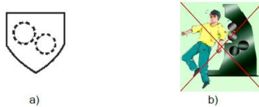
Figure 2. a) A pictogram of clothing suitable for protection against movable parts of machines; (b) An example of unsuitable protective clothing
