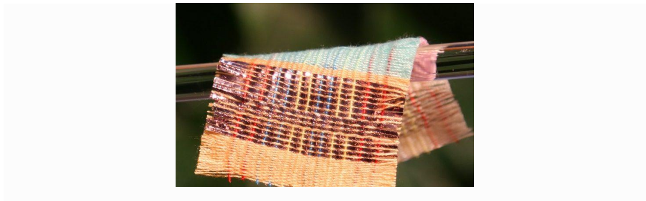
Figure 8. Photovoltaic fabric developed in the Georgia Institute of Technolog.
