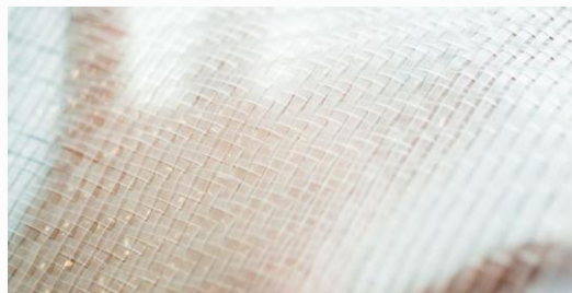
Figure 6. Photovoltaic fabric produced by Imec.
