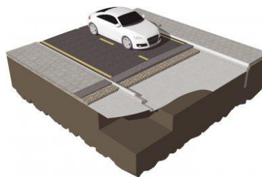
Photo 11. Geotextile display in road construction
