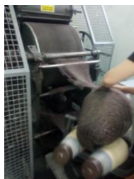
Picture 10: worker who is winding flor on the wooden cone - roller
