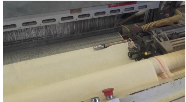
Image 5. Weaving fabrics of various densities and fineness on debauchery
