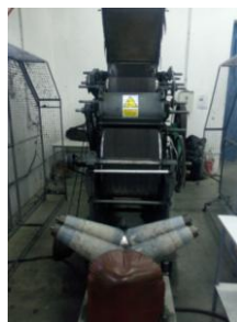
Picture 8: Appearance of a conus-picking machine
