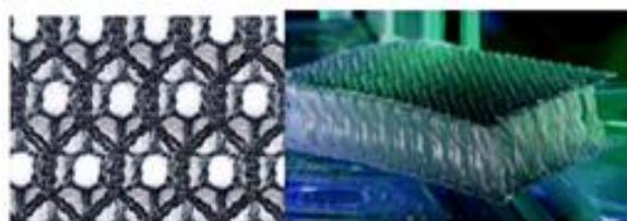
Image 2. Examples of spaces in knitwear with closed and opened structure
