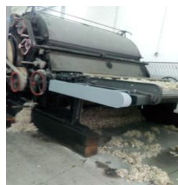
Picture 2: Display of the waste wool under the picking machine
