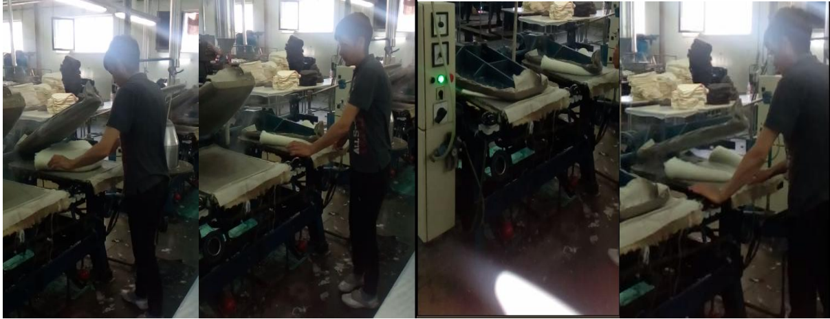
Pictures 21,22,23,24: Placement of the cone on the felt-machine (felting)
