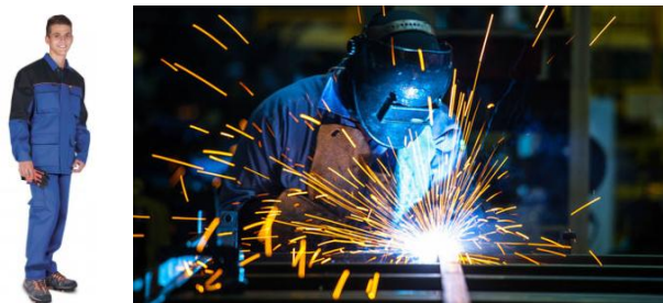
Figure 9. Protective clothing for welding
