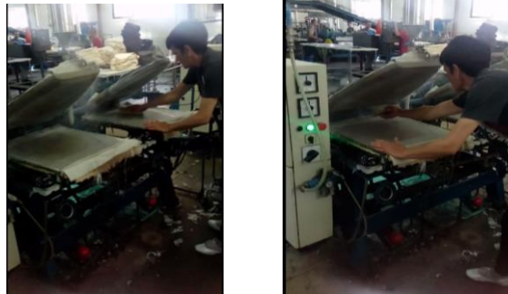
Pictures 16,17: Cleaning of the working surface
